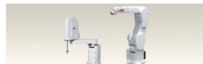
Roboter: SCARA, Knickarm
